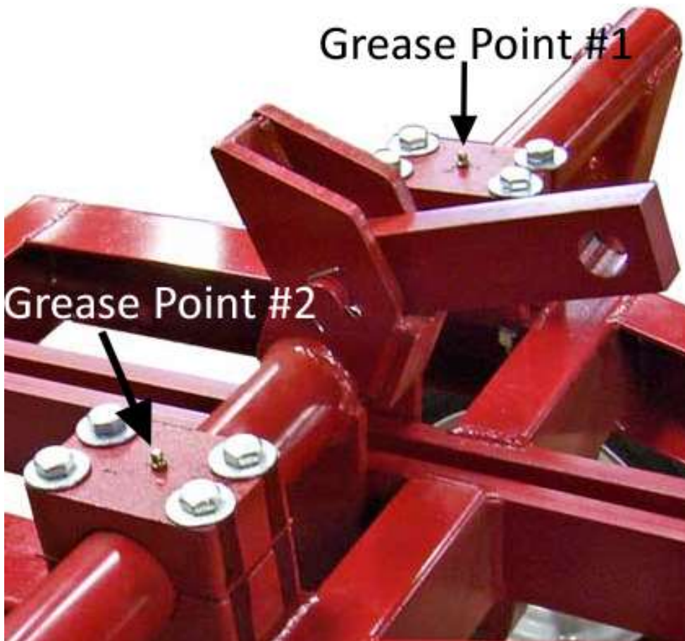
Figure 16: Packer Wheel Axle Grease Points
