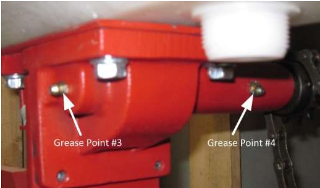
Figure 17: Seeder Casting Grease Points
