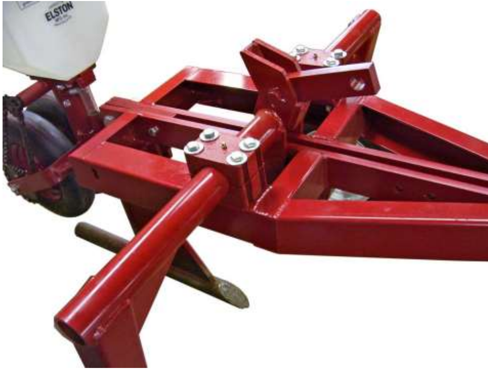
Figure 7: Image of Axle Assembly as Installed
