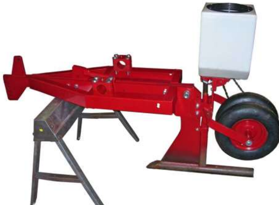
Figure 4: Frame and Seeder/Knife Assembly Mounted Together
