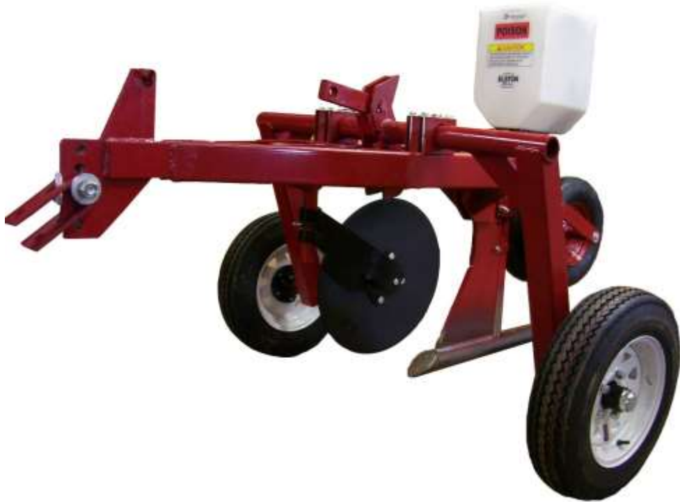
Figure 8: 18" Coulters Assembly as Installed
