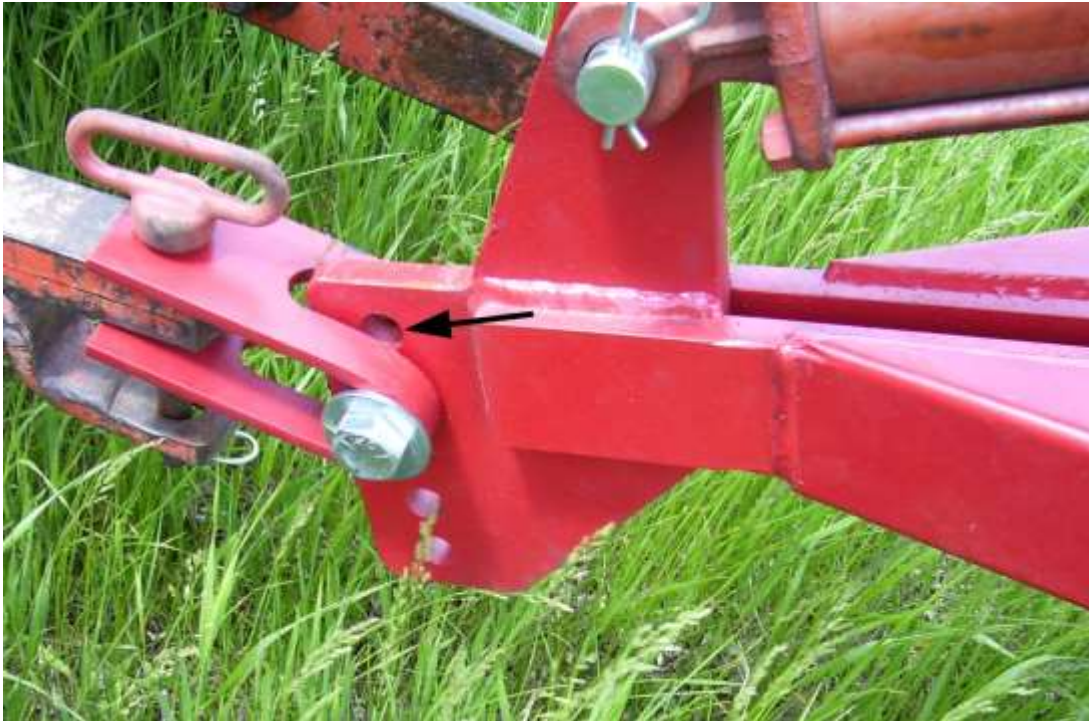
Figure 12: Changing Hitch Clevis on the Frame
